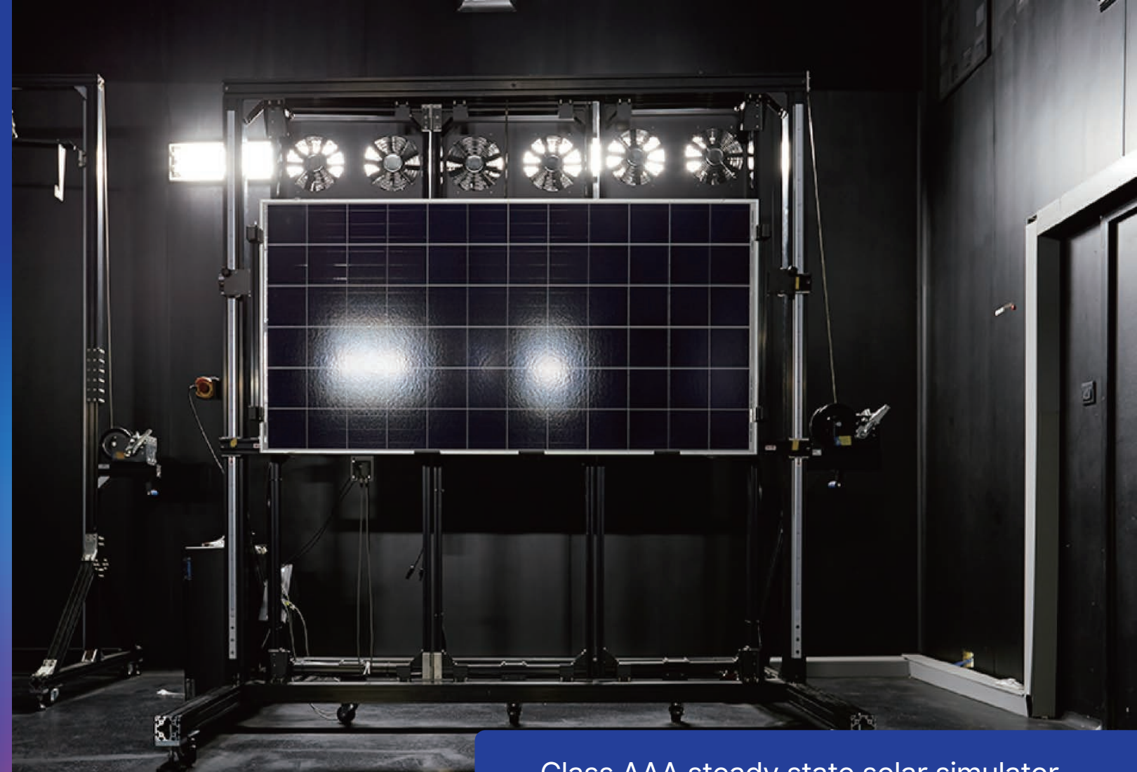
Class AAA steady state solar simulator
